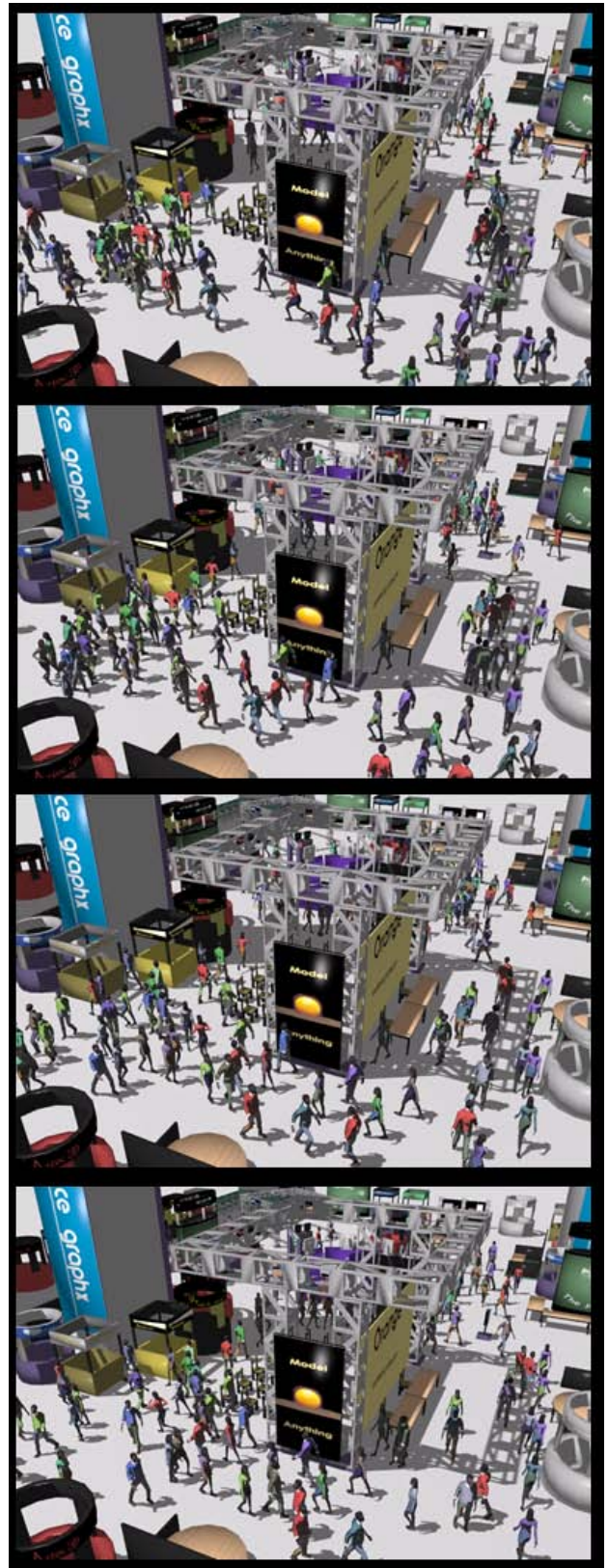
Figure 7: Sequence of 4 snapshots from Tradeshow demo. The environment contains 511 booths with 110K polygons. The agents move toward different booths and avoid each other using link bands.
